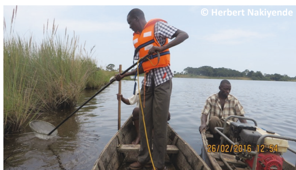
Image 2. Electro-fisher being used to sample fish in lake Kanyanja.
